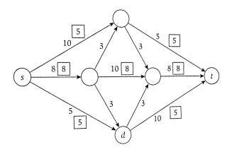
What is the value of this flow? Is this a maximum (s, t) flow in the graph? What is the minimum s-t cut in this graph?
