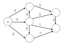
5. [10 pts] Consider the weighted directed graph above. Draw 1) the shortest path tree rooted at v that would be found by Dijkstra's algorithm and 2) the shortest path tree rooted at v that would be found by the Bellman-Ford algorithm. (You must show your work for partial credit.) Which, if any (or both), of these trees give the correct shortest paths?
