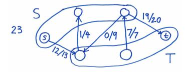
net flow across cut: f(S, T) = (12 + 0 + 19) - (1 + 7) = 23capacity of cut: c(S, T) = 13 + 9 + 20 = 42 $f(S, T) \le c(S, T)$  for every cut (S, T)
