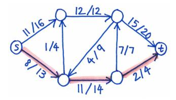
the flow can be increased by 2 units along the path
