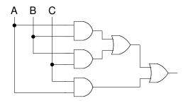
Take 0 for A, the value 1 for B, and 0 for C. What does the circuit compute?
