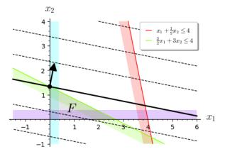
Starting at  $(x_1 = 0, x_2 = 0)$ , the simplex method pivots to an adjacent corner of the feasible region that has a better optimum.
