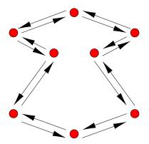
The triangulation is also stored in a doubly connected edge list.
