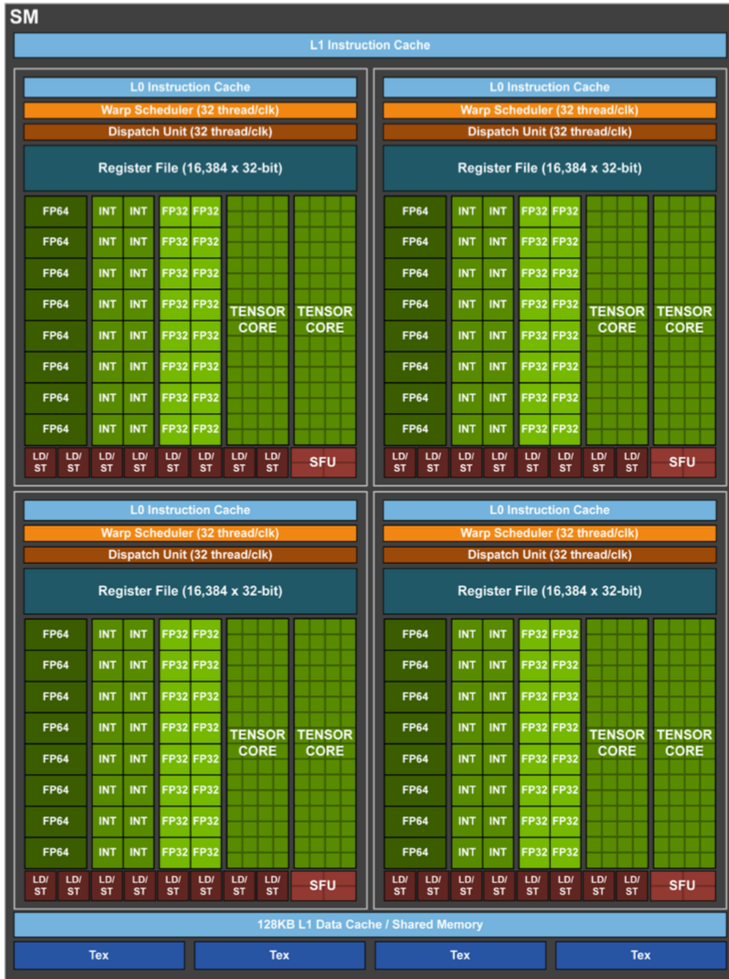
Fig. 6.38: The Volta Streaming Multiprocessor, picture from the NVIDIA Volta Architecture white paper.
