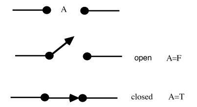
A signal can go from left to right through the switch when it is closed, and no signal can go through when the switch is open. We choose to designate a switch by a label such as A above and we let A = T correspond to the closed switch position (T for "transmit" if you like!) and we let A = F when the switch is in the open position (F = T = not transmit).
