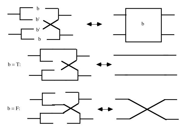
In the figure above we have indicated the middle switch by a box with the label b, and we have illustrated how the two states of the switch correspond to parallel and crossed lines. By simplifying the symbolic logic solution to the three switch light problem, we have invented a useful new switch. Lets call this switch, as shown above, the *crossover switch*.
