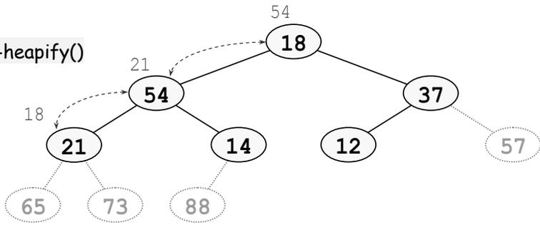
Five more exchanges, followed by calls to *fixHeap()*, complete the transformation from a heap to a sorted array.
