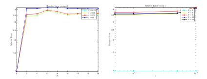
• In this resonant configuration, the IIO algorithm again displays a spectral rate of convergence as *N* is refined, while the DNO approach delivers completely unacceptable results.
