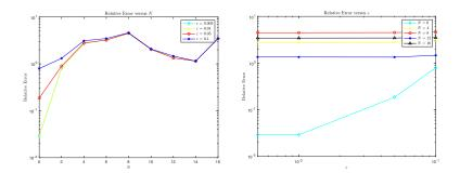
In this nearly resonant configuration, while IIO algorithm displays a spectral rate of convergence as N is refined, the DNO approach does not provide results of the same quality.
