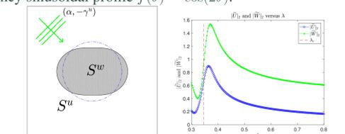
(a) Cross-section of a silver nanorod ( $S^w$ ) shaped by  $r = \bar{g} + \varepsilon \cos(2\theta)$  housed in a vacuum (dielectric) under plane ( $S^u$ ).
