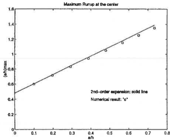
Fig. 9. Run-up at the place of the collision: (o) numerical; solid line: second-order expansion.
