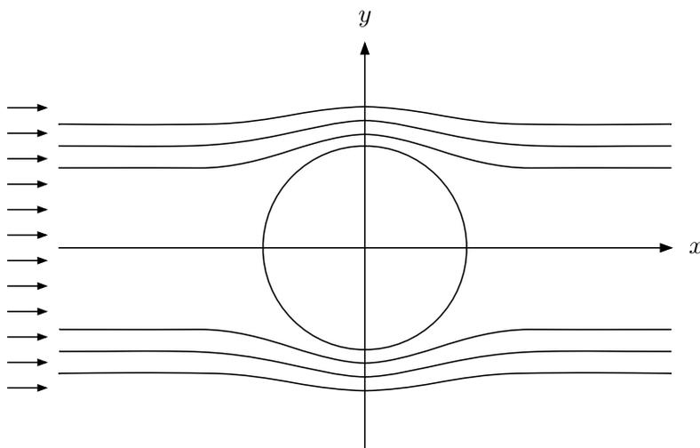
Figure 1.3: Elementary flow III, flow past a cylinder.
