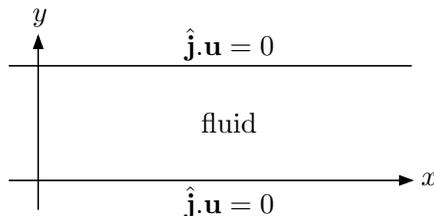
Figure 1.3: Fluid in a periodic channel.
