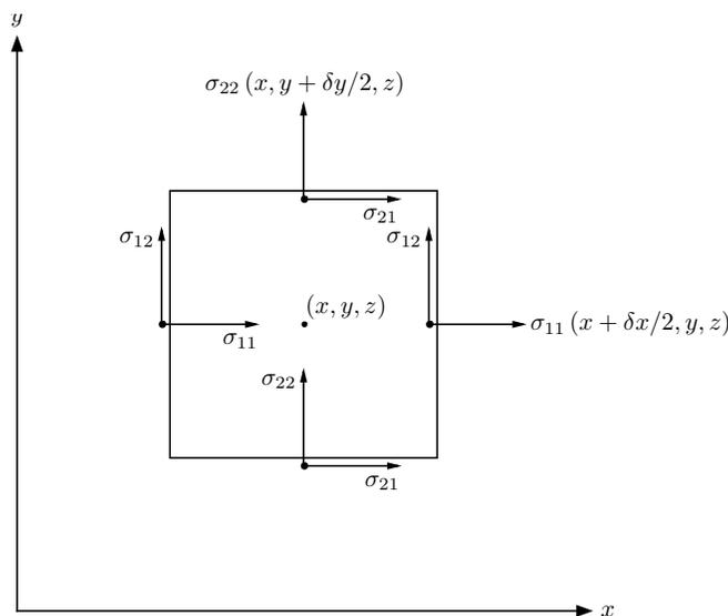
Figure 1.2: Stress on a fluid element.
