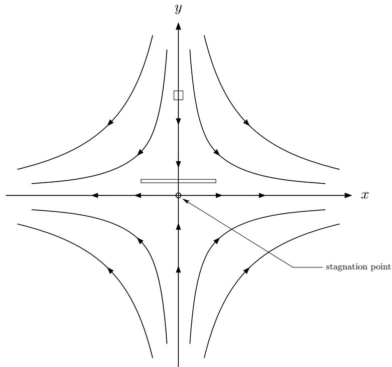
Figure 1.2: Elementary flow II, uniform strain.
