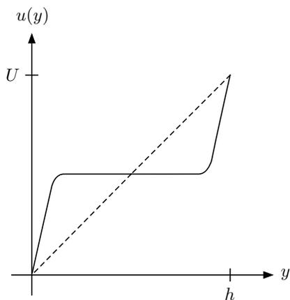
Figure 2.1: Expected turbulent Couette flow profile.
