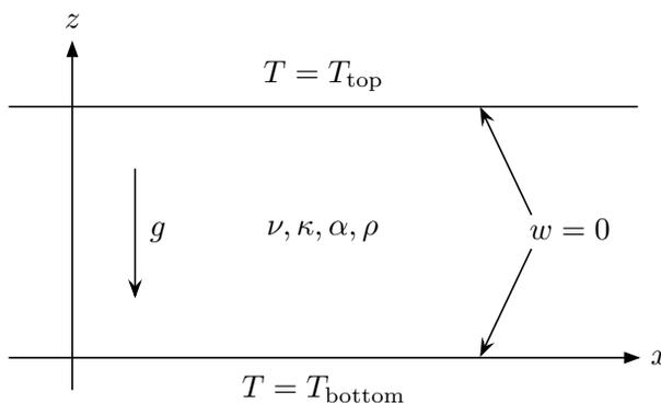
Figure 3.1: Setup for Rayleigh-Benard convection.
