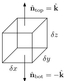
Figure 2.3: Normal forces on a fluid element.
