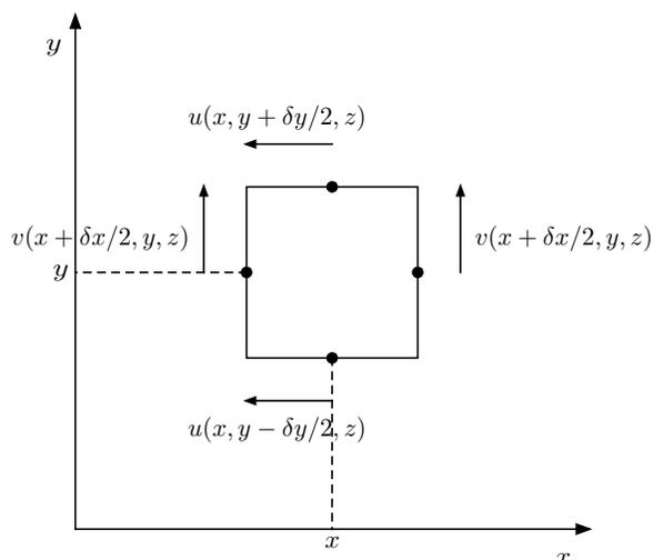
Figure 3.2: Computing angular velocity.
