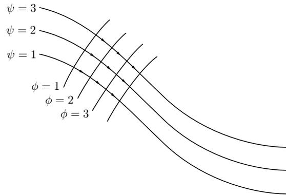
Figure 2.1: Level sets of  $\phi$  and  $\psi$  in potential flow.
