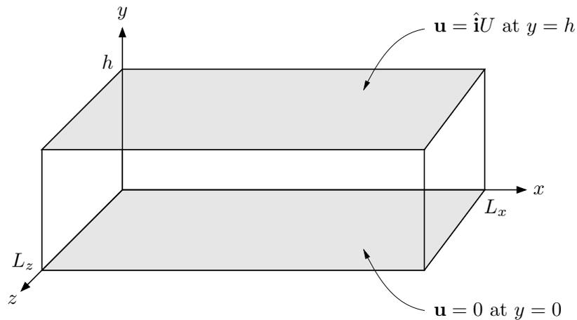
Figure 1.1: Setup for plane Couette flow.
