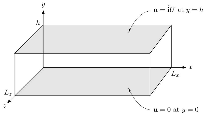
Figure 0.1: Setup for plane Couette flow.
