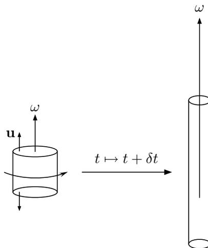
Figure 2.1: Vortex-stretching in a fluid element.
