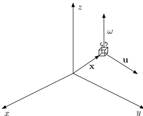
Figure 3.1: Vorticity of a fluid element.
