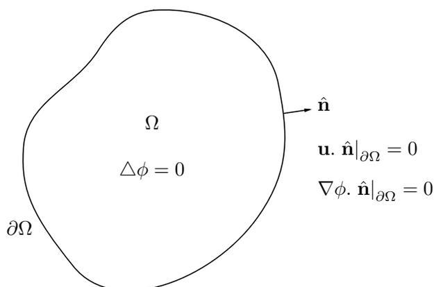
Figure 1.3: Laplace's equation with Neumann boundary condition.
