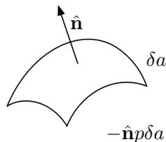
Figure 0.2: Force on an infinitesimal area  $\delta a$ .
