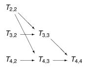
For n = 4, with 3 processors, it takes 3 steps to compute the table. The speedup is 6/3 = 2. Each path leading to  $T_{4,4}$  has two edges or three nodes. So, the length of the critical path is 2.
